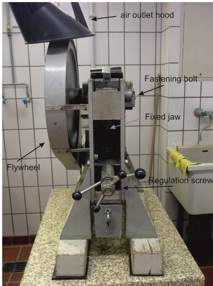
Fig. 2: The jaw-crusher and important components. Viewed from the front.
