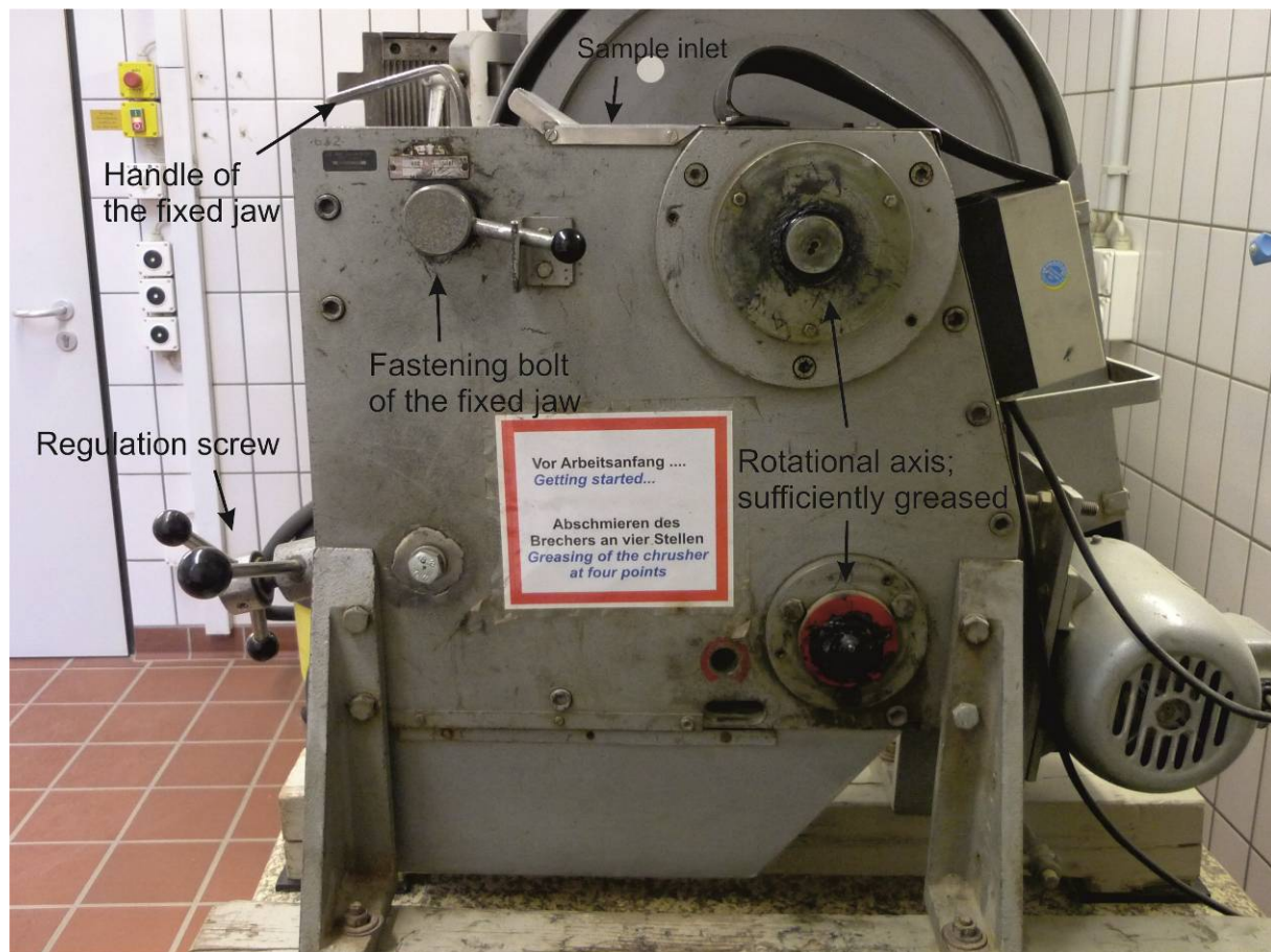
Fig. 1: The jaw-crusher and important components. Viewed from the side.
