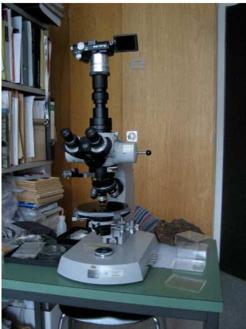
Fig. 3: Petrographic microscope for final selection.
