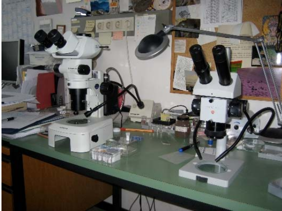
Fig. 2: Binocular microscopes. Left: Scope for pre-selection; Right: Scope for producing platinum capsules and transferring grains into capsules.
