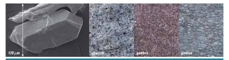
selFrag Lab – the first commercial High Voltage (HV) pulsed power laboratory equipment for selective fragmentation. Very short pulsed HV-discharges applied to solids under water cause the material to disaggregate along grain boundaries, inclusions or inhomogeneities. The highly selective fragmentation process of selFrag Lab liberates morphologically intact minerals while minimizing the production of undesired fines.
