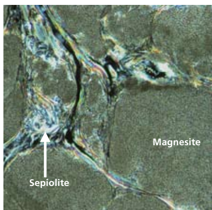
Magnesite ( \text{MgCO}_3 ) ore with sepiolite intergrowth
