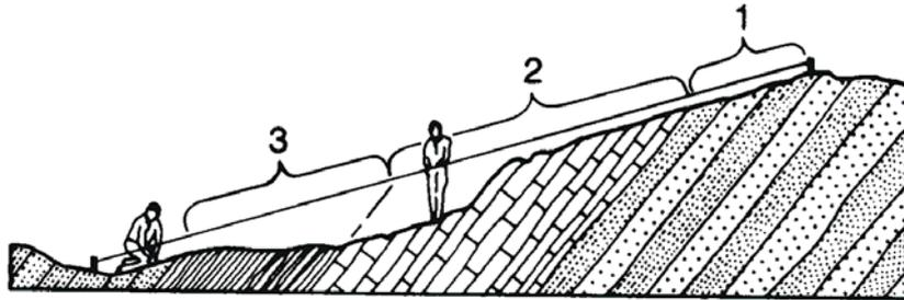
**Fig. 2.18.** Measurement of strata on a slope by reference to a stretched tape. Note the projection of contact between units (2) and (3) to the tape (from Compton, 1962). (Reproduced by permission of Wiley.)
